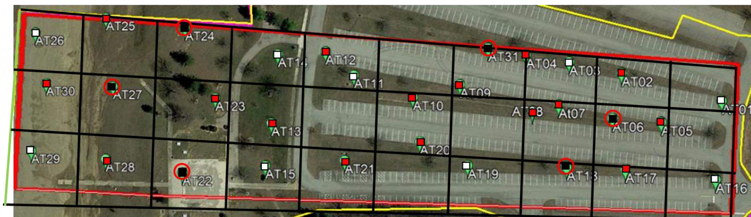
Figure 4.83: Positions of the Targets as GCPs for the 9 GCPs 3D point Cloud
