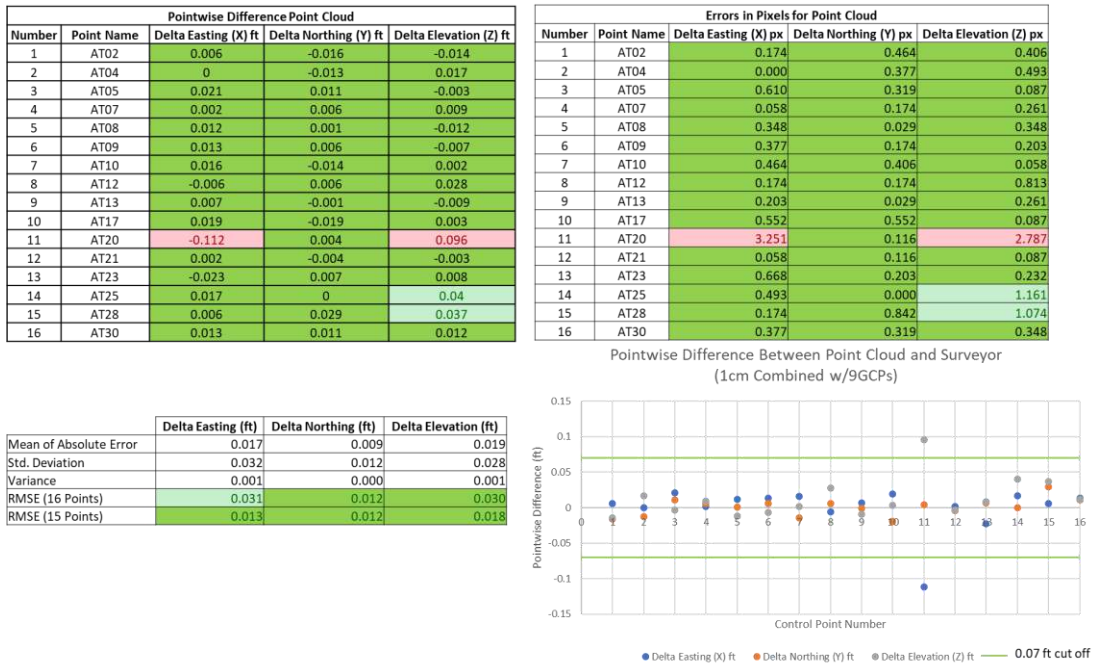
Figure 6.10: Error Data Compiled for the 3D Point Cloud Generated Using the 1cm/px Grid Dataset with 9 GCPs
