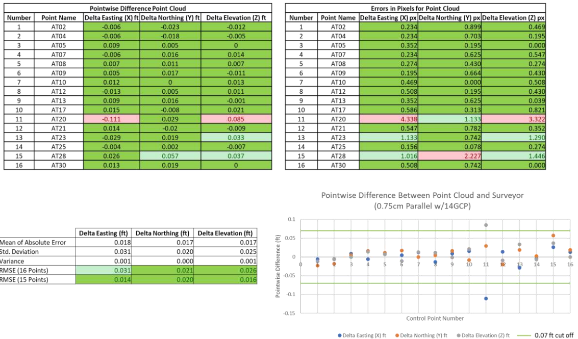
Figure 6.2: Error Data Compiled for the 3D Point Cloud Generated Using the 0.75cm/px Parallel Dataset with 14 GCPs
