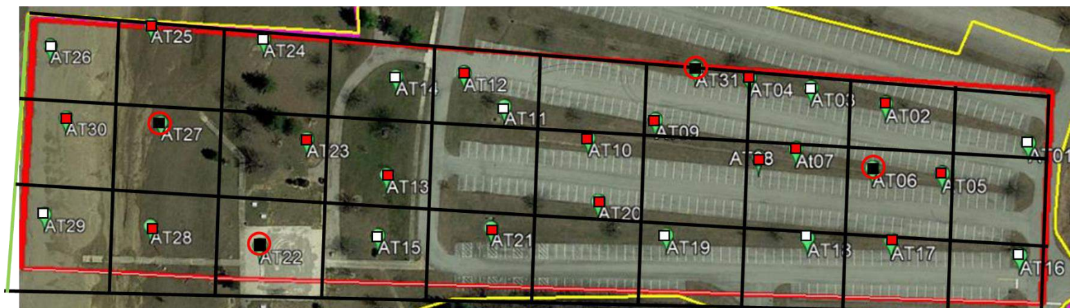
Figure 4.82: Positions of the Targets as GCPs for the 11 GCPs 3D point Cloud
