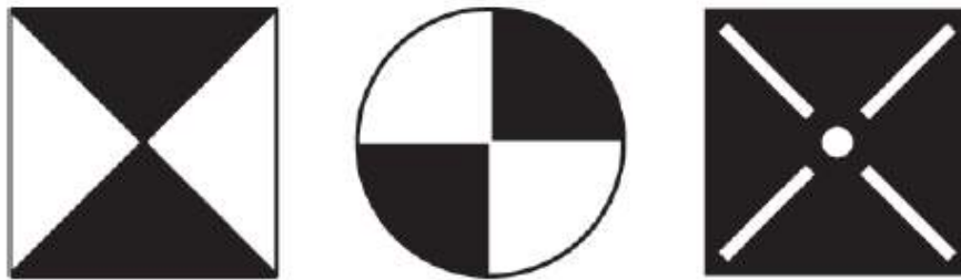
Figure 2.39: Examples of GCP Target Shapes and Designs [41]
