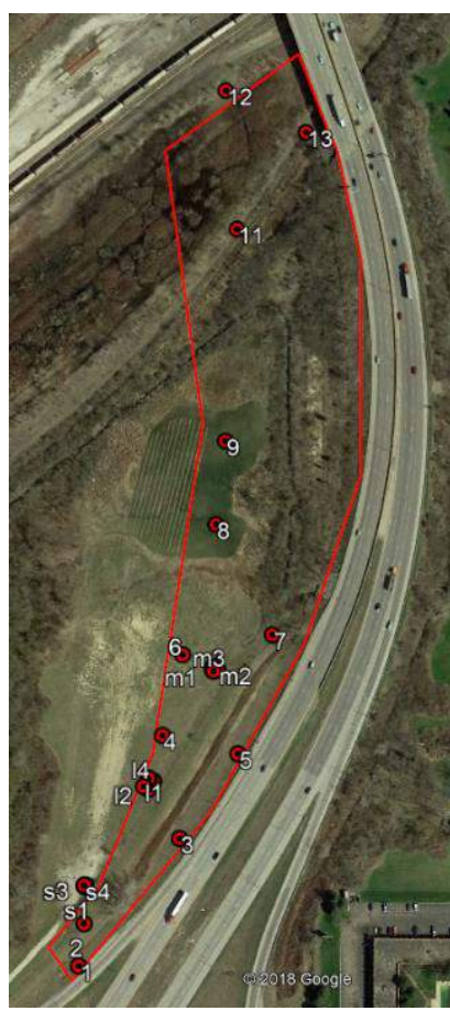
Figure 4.62: Locations of the GCPs Marked on the Region Mapped for the i75 Construction Site Case Study
