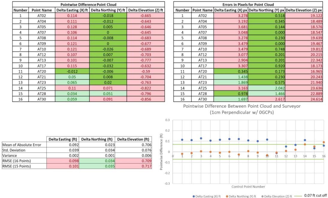
Figure 6.17: Error Data Compiled for the 3D Point Cloud Generated Using the 1cm/px Perpendicular Dataset with 0 GCPs
