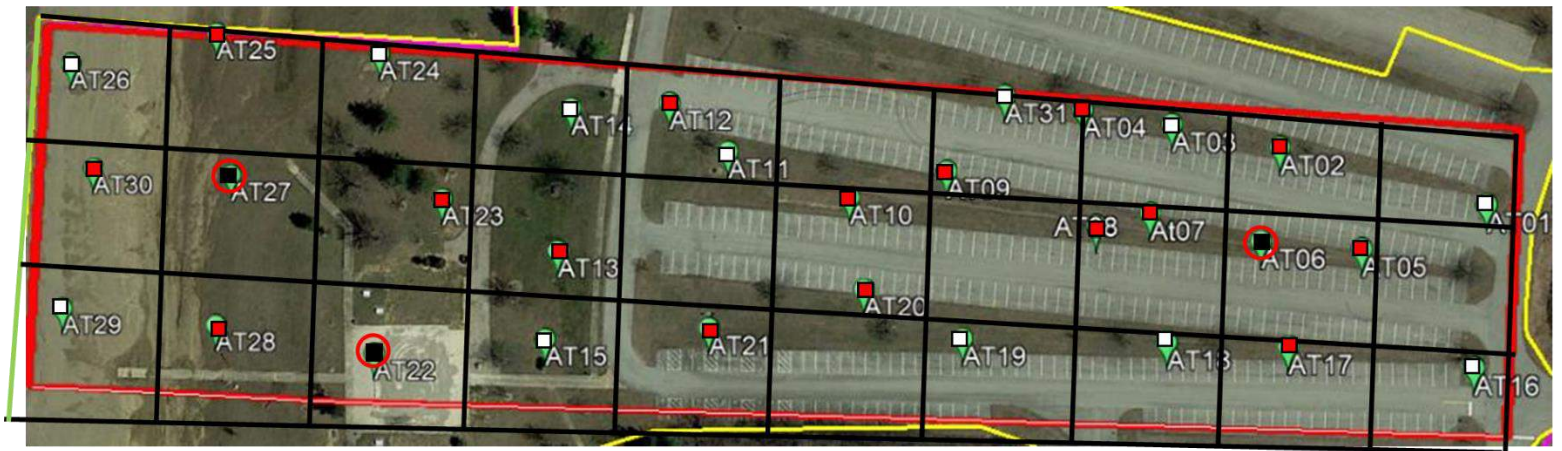
Figure 4.81: Positions of the Targets as GCPs for the 12 GCPs 3D point Cloud
