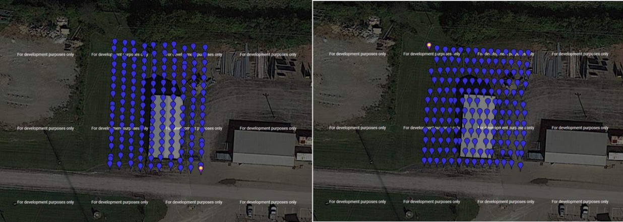
Figure 3.49: Flight Pattern Experiment Image Locations; Left: Parallel Dataset (Flight 1), Right: Perpendicular Dataset (Flight 2)
