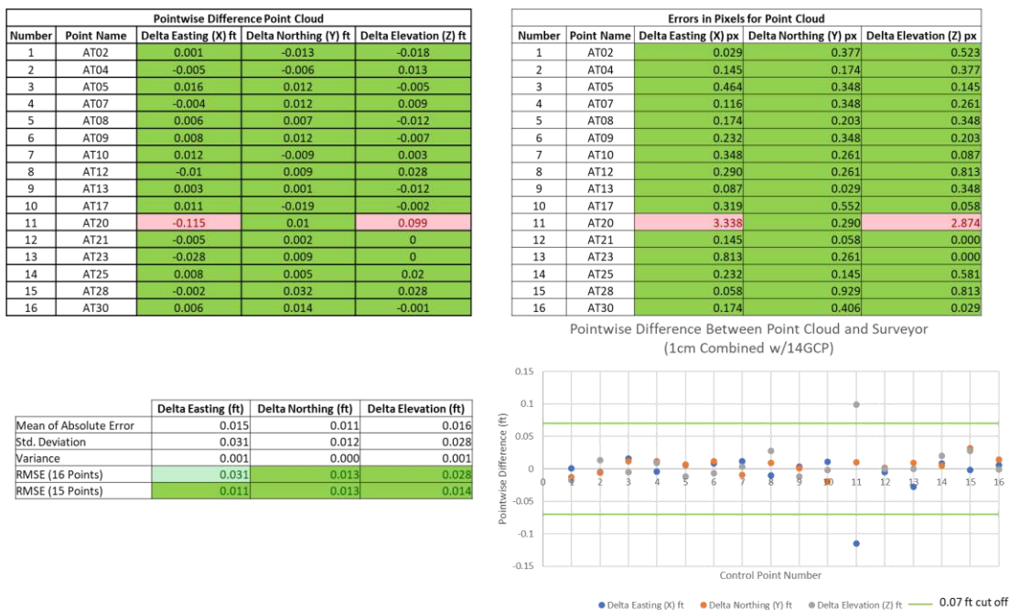
Figure 6.7: Error Data Compiled for the 3D Point Cloud Generated Using the 1cm/px Grid Dataset with 14 GCPs
