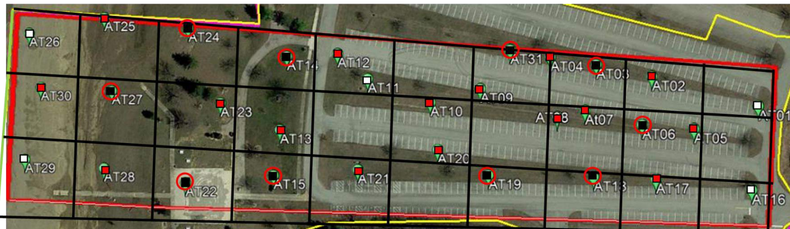
Figure 4.85: Positions of the Targets as GCPs for the 5 GCPs 3D point Cloud
