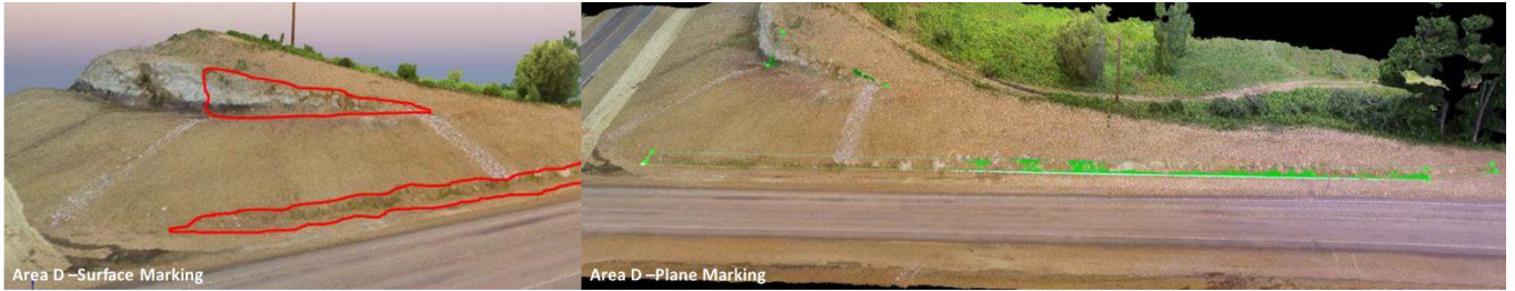
Figure 4.14: 3D Point Cloud of SR266 Area D with Pre-splits Marked; Left: Surface Marking, Right: Plane Marking
