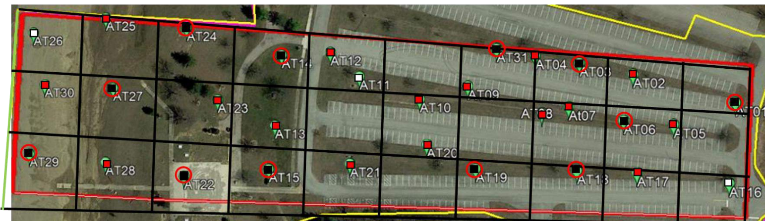
Figure 4.86: Positions of the Targets as GCPs for the 3 GCPs 3D point Cloud
