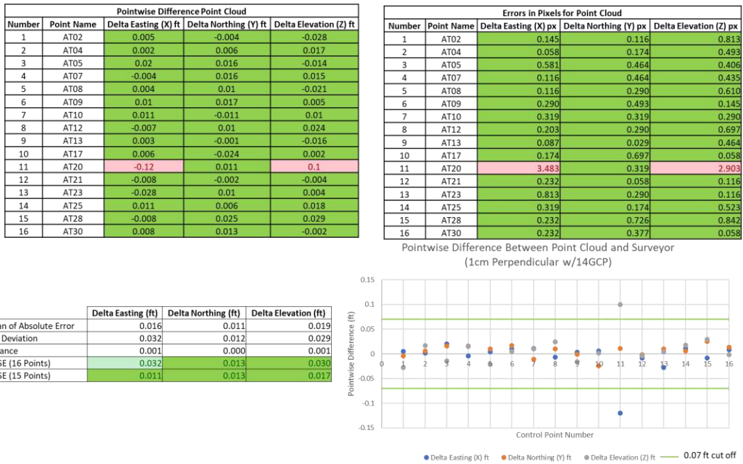
Figure 6.16: Error Data Compiled for the 3D Point Cloud Generated Using the 1cm/px Perpendicular Dataset with 14 GCPs
