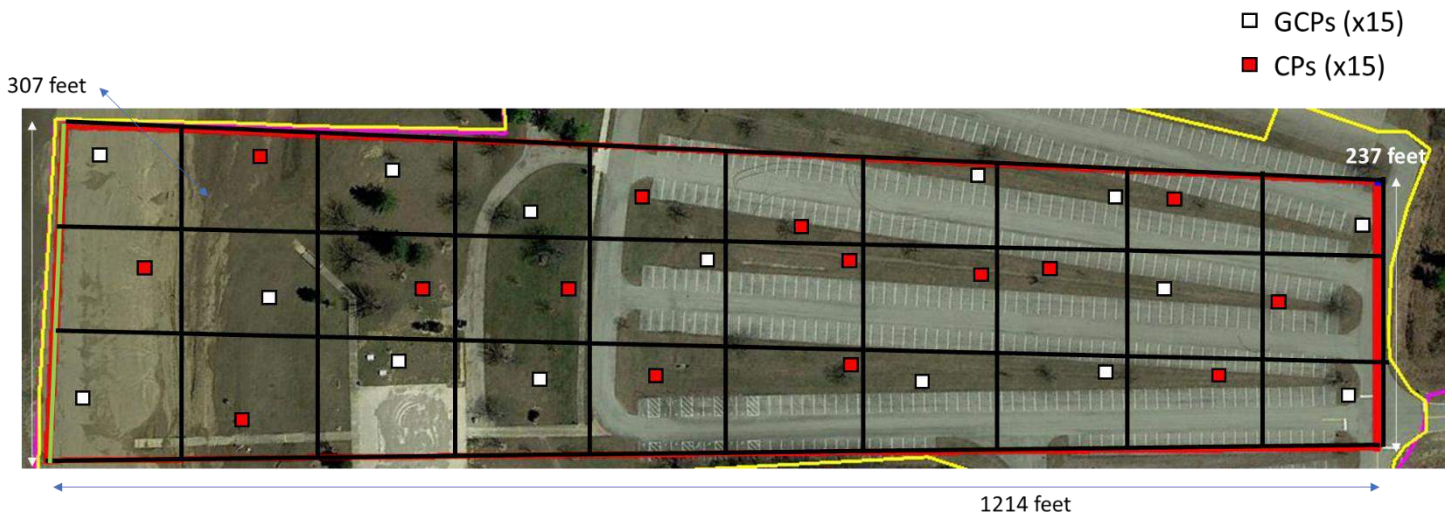
Figure 4.75: Map of the Region Mapped with Vinyl Targets Designated as GCPs and Check Points
