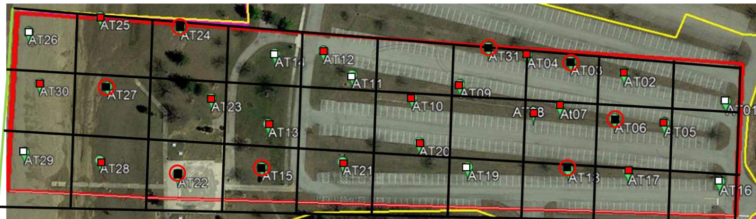
Figure 4.84: Positions of the Targets as GCPs for the 7 GCPs 3D point Cloud
