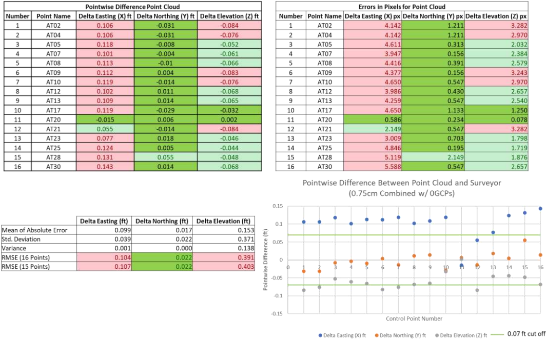
Figure 6.3: Error Data Compiled for the 3D Point Cloud Generated Using the 0.75cm/px Grid Dataset with 0 GCPs
