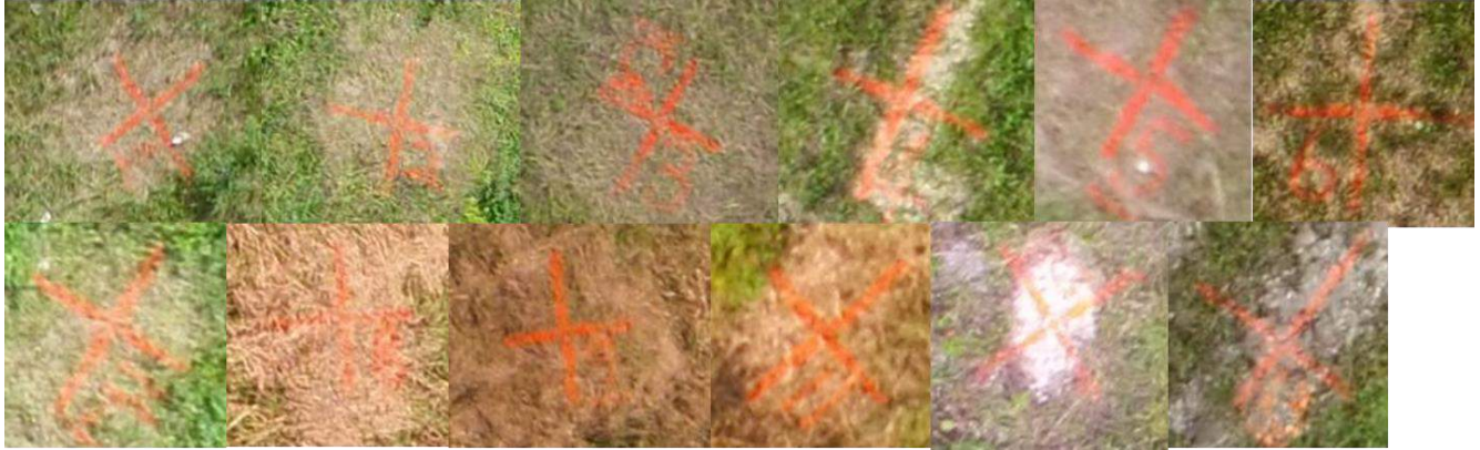
Figure 4.63: Images of the GCPs Marked on the Field for the i75 Construction Site Case Study
