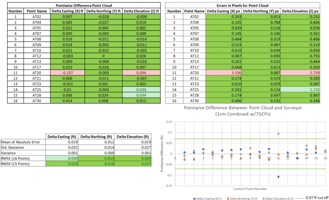
Figure 6.11: Error Data Compiled for the 3D Point Cloud Generated Using the 1cm/px Grid Dataset with 7 GCPs
