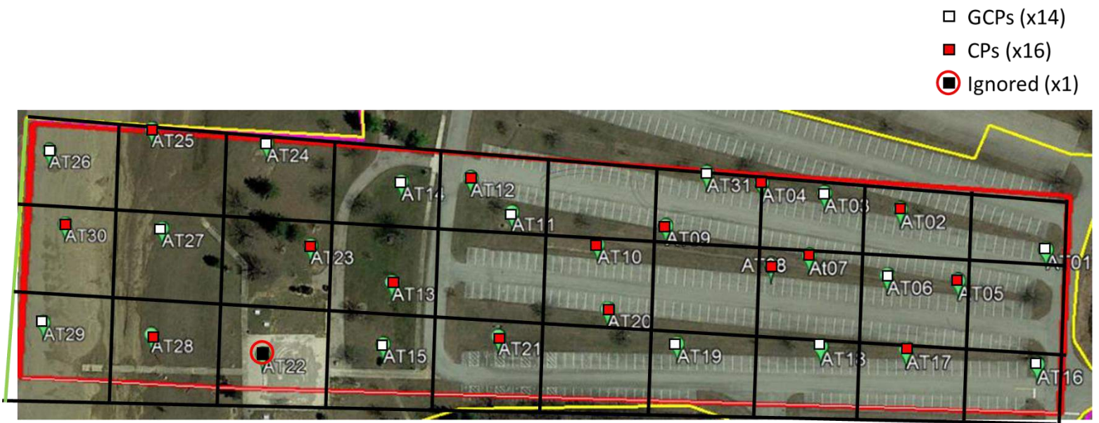
Figure 4.76: Actual Positions of the Vinyl Targets and Targets Selected as GCPs and Check Points
