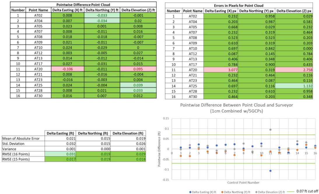
Figure 6.12: Error Data Compiled for the 3D Point Cloud Generated Using the 1cm/px Grid Dataset with 5 GCPs
