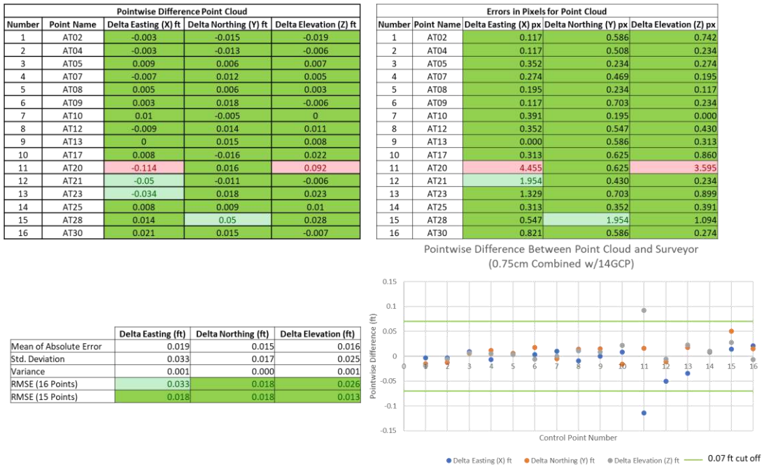
Figure 6.1: Error Data Compiled for the 3D Point Cloud Generated Using the 0.75cm/px Grid Dataset with 14 GCPs
