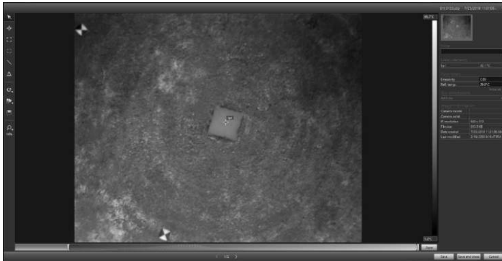
Figure 2.28: FLIR Tools Interface to Measure Temperature Using Spot Measurement Tool
